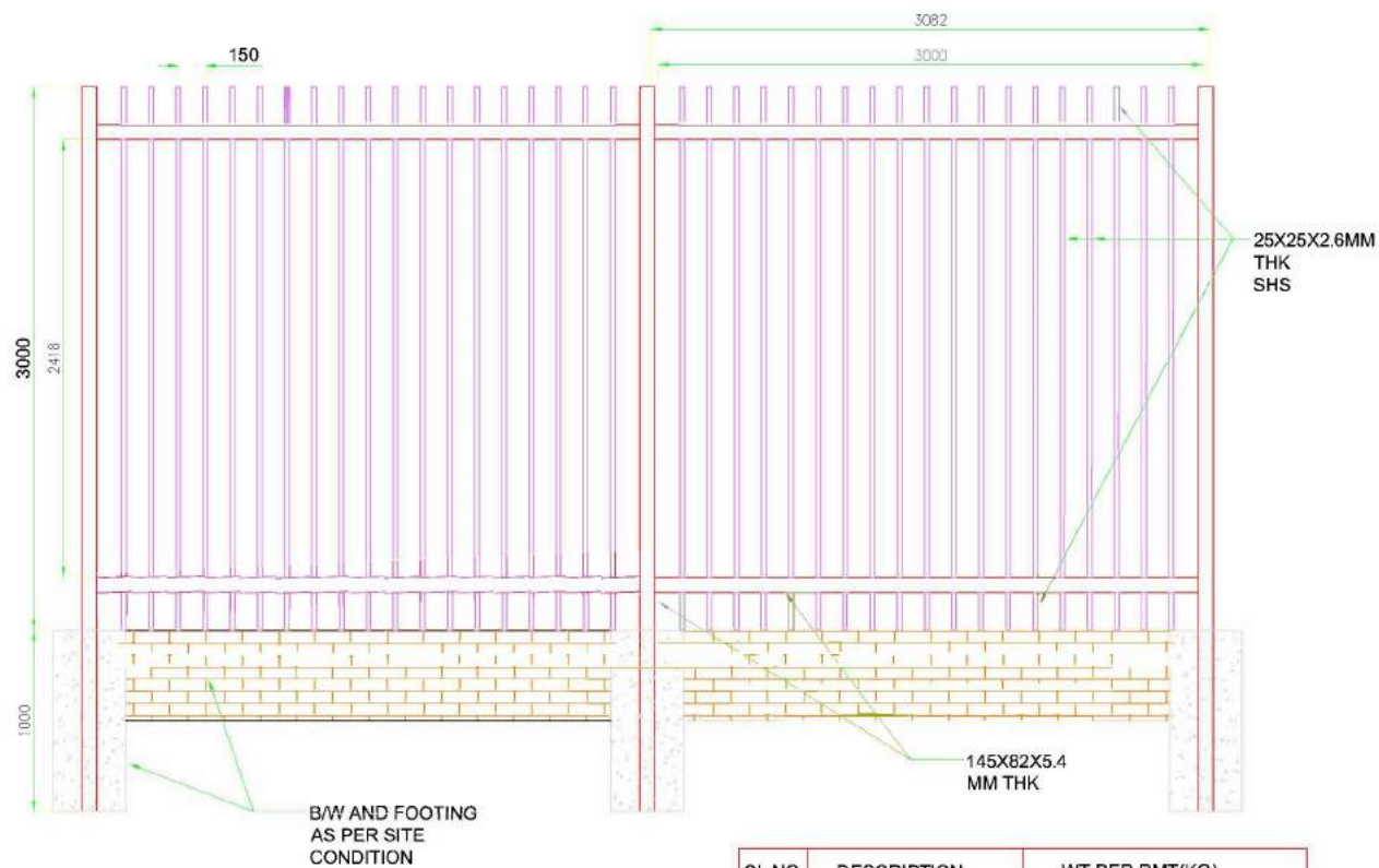
BOUNDARY FENCE: AGIRAILING-066 HEIGHT : 10 FT
